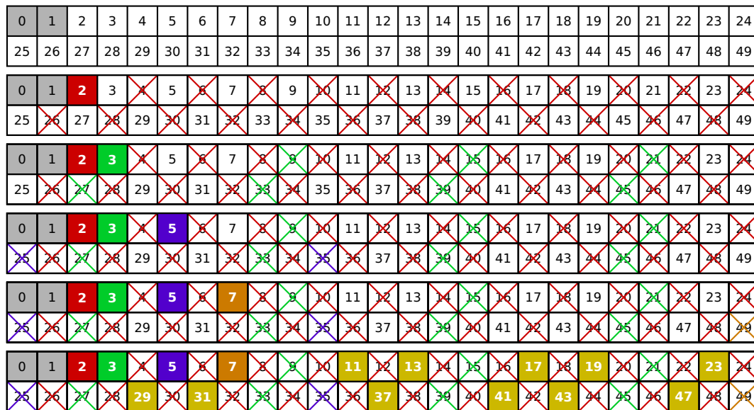
Figure 4.7: Iteration steps when the sieve of Eratosthenes is used to determine the prime numbers below 50. For details see the main text.
